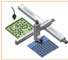
Vision System for Pick & Place Application
